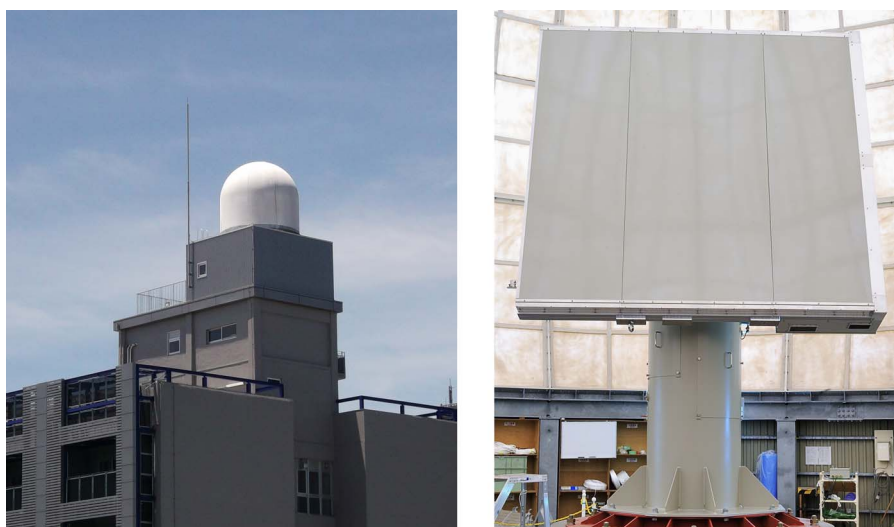
Fig. 3. Photographs of the PAWR at Suita Campus, Osaka University (cf., [42, Fig. 10]). (Left) PAWR at the top of the Electrical Engineering Department building at Osaka University. (Right) Antenna of the PAWR system inside the Radar Dome.
