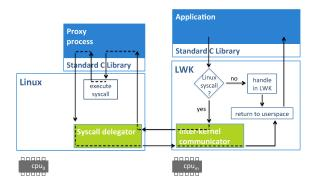
Figure 1: Overview of the proxy model and the system call delegation mechanism.
