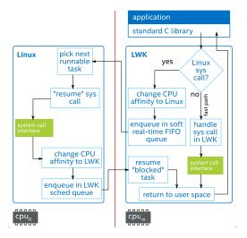
Figure 3: System call execution using the Evanescence mechanism.
