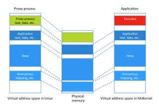
Figure 2: Unified virtual address space of the proxy process on Linux and the corresponding application on the LWK.
